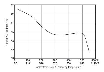
Hardening temperature: 1030°C / 1886°F Specimen size: square 20 mm
