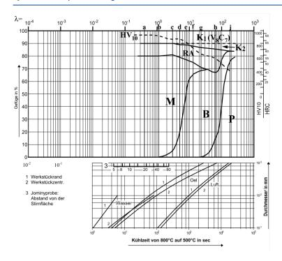
HV10... Vickers Hardness K... Carbide
